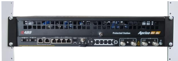
Rack mounted Aprisa SRi Protected Station without duplexer
